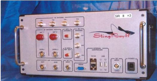
An example of equipment that can be used to set up a rogue cell site. The entire set-up can fit in a van.
